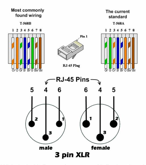
With 5 pin XLR you do not use XLR pins 4 and 5. Pins 1, 2 and 3 are connected as above.
